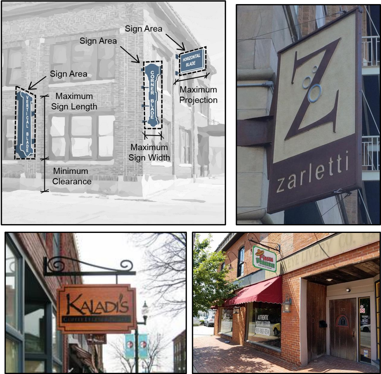
Figure 4.16-B: Projecting sign measurement locations and examples
