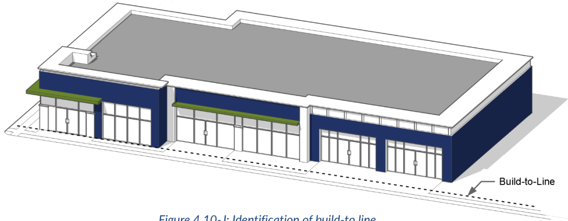
Figure 4.10-J: Identification of build-to line
