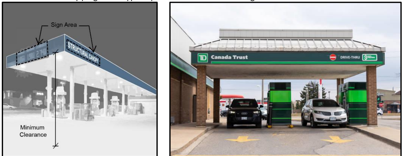
Figure 4.16-H: Structural canopy sign measurement locations and sample signs
