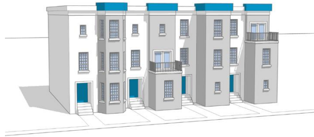
Figure 10-B: Façade articulation example
