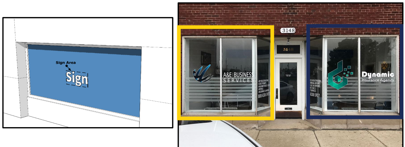
Figure 4.16-D: Window sign measurement locations and samples
