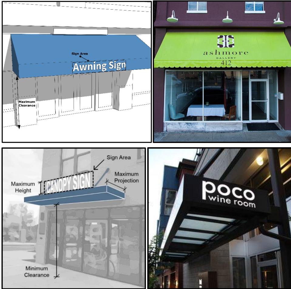
Figure 4.16-A: Awning and Canopy sign detail
