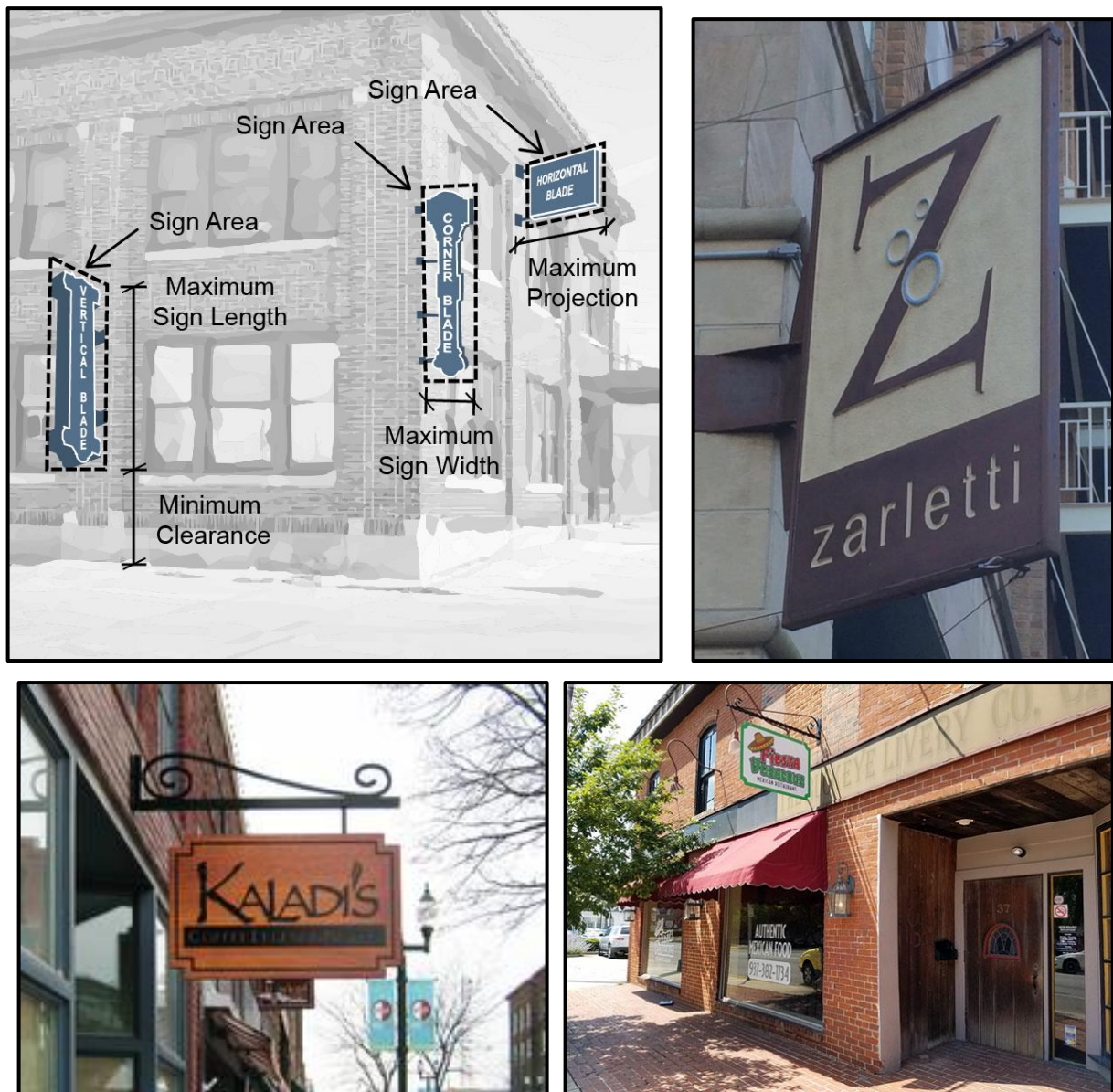
Figure 4.16-B: Projecting sign measurement locations and examples
