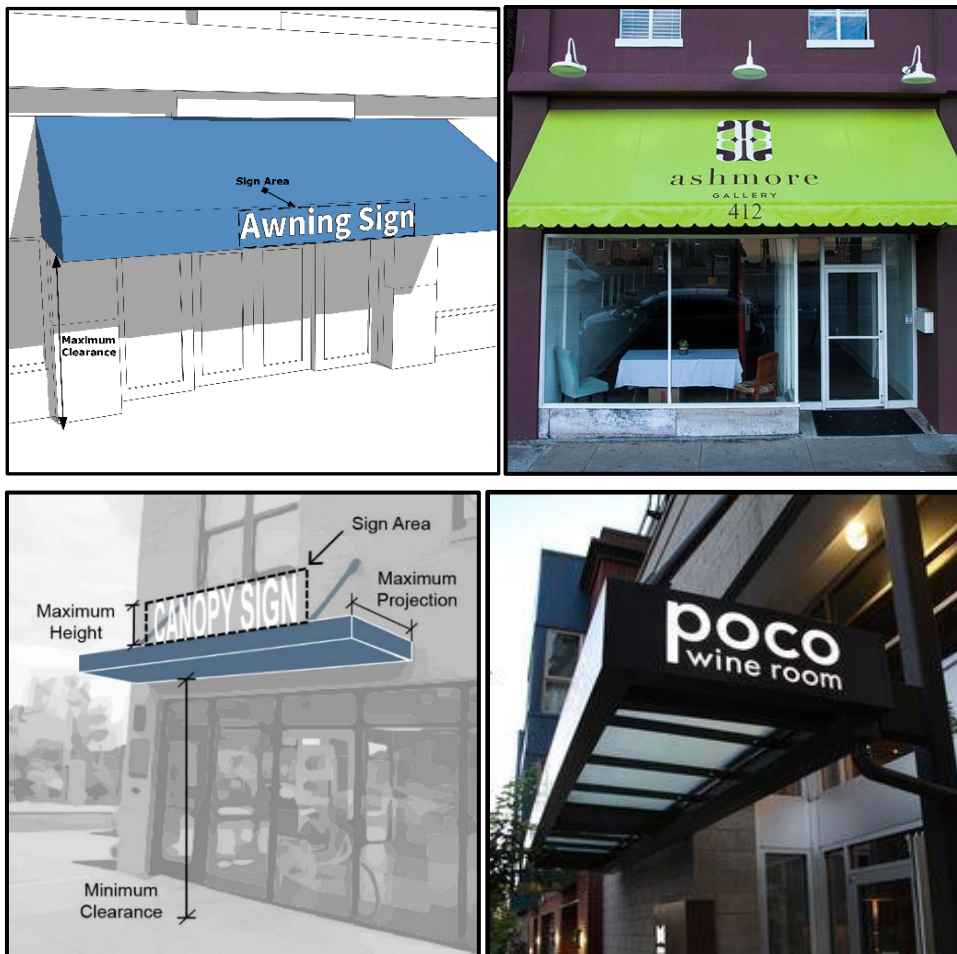
Figure 4.16-A: Awning and Canopy sign detail
