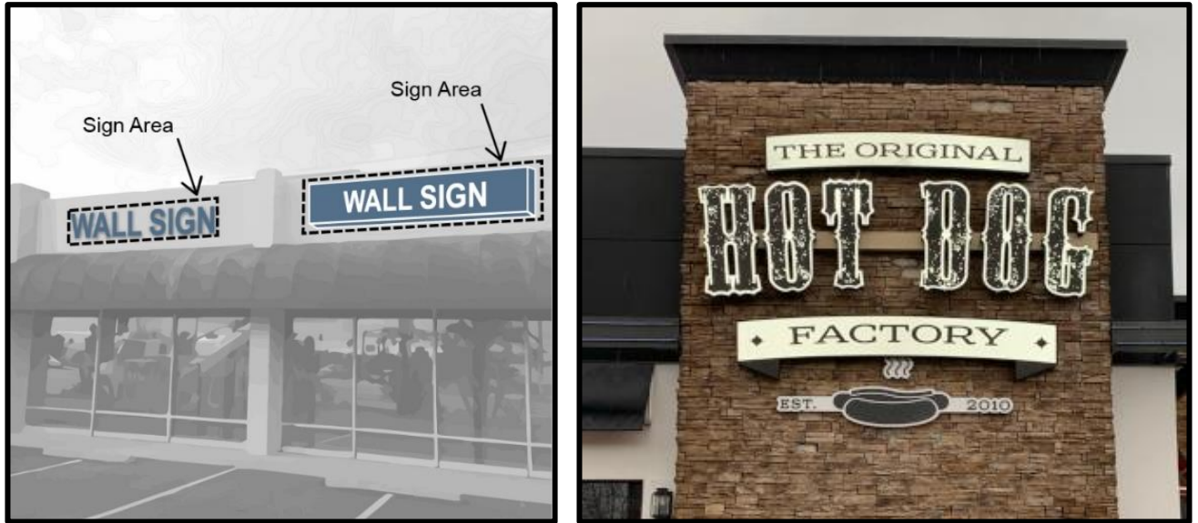
Figure 4.16-C: Wall sign measurement locations and sample
