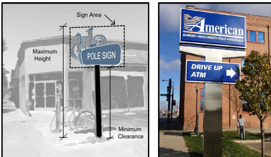
Fig. 4.08-G: Pole sign measurement locations and sample sign
